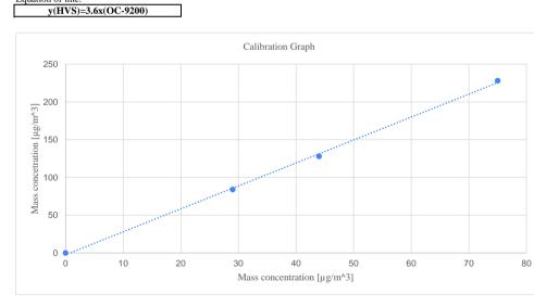
In-house method in according to the instruction manual: The OC-9200 was compared with a calibrated HVS; the result has been used to calculate the scale factor and correlation coefficient between the two equipment. **The filter papers are weighted by HOKLAS laboratory (HPCT Litimed)**
